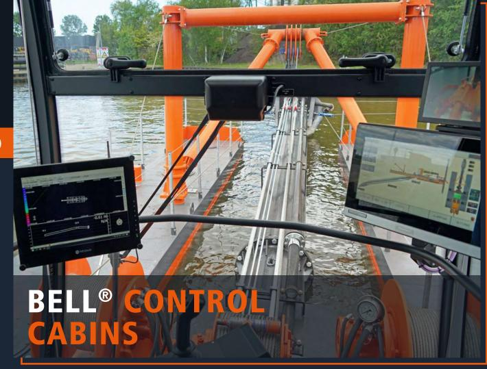
A climate controlled, spacious cabin with comfortable chair and windows 180 degrees from left to right ensures maximum operator comfort. The dredger is controlled with two joysticks and all aspects of the dredging process are monitored on two tablet screens. A rear view camera is installed on the backside of the cabin.
